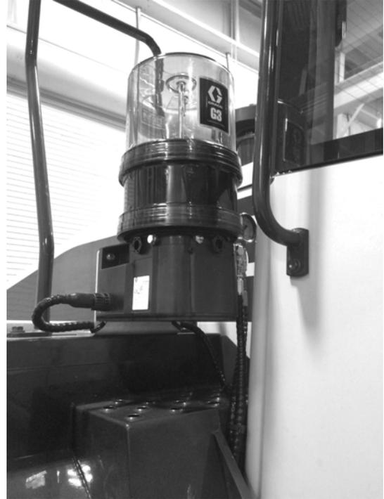
**FIG. 46: Deck Plate Mounting**
