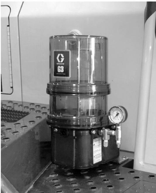
**FIG. 45: Deck Plate Mounting**
