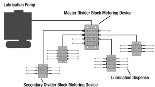
**FIG. 16: Series Progressive System Typical Installation**
